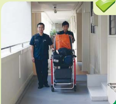
Ambulance crew and wheel chair bounded person requires at least 1.2m clear width for access.
